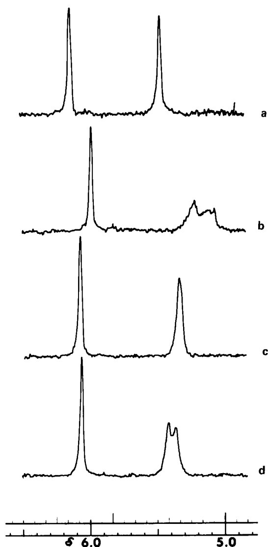
Fig. 1. 60 MHz nmr spectra of the vinylic regions of TCNE adducts a) 12j , b) 12d , c) 12e and d) 12f .
